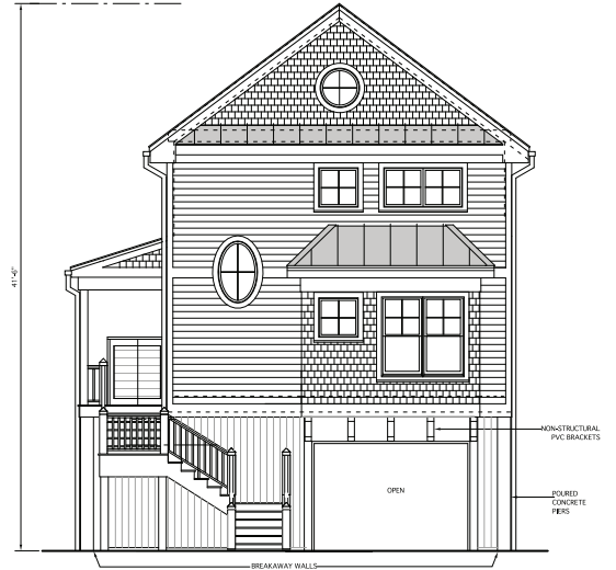
ELEVATION TOWARDS PARKING SCALE: 1/4" = 1'-0"
